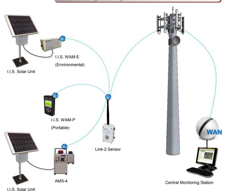
The Area Radiation monitor transmits data to a Link-2 base station from up to a mile away. Each base station can handle up to 8 Radiation monitors, allowing you to monitor multiple facilities and areas by using cellular tower technology to transmit the data back to your central monitoring location.
